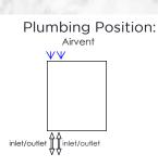
All Dimensions are in mm Max.Working Pressure: 10 Bar Max.Working Temperature: 95° C Inlet / Outlet : 1/2" BSP Fuel Type: E
