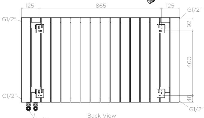
All Dimension are in mm Max.Working Pressure = 10 Bar Max.Working Temperature=95° C Inlet / Outlet : 1/2" BSP
