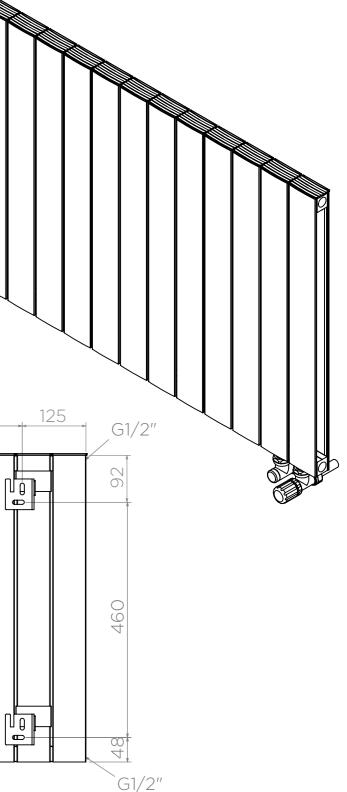
All Dimension are in mm Max.Working Pressure = 10 Bar Max.Working Temperature=95° C Inlet / Outlet : 1/2" BSP
