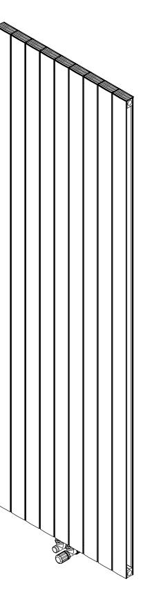
All Dimension are in mm Max.Working Pressure = 10 Bar Max.Working Temperature=95° C Inlet / Outlet : 1/2″ BSP
