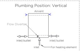
When mounting vertically, please observe that the collector fitted with a flow diverter is mounted at the bottom. This can be verified by visually checking or by referring to the installation diagram.
