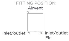
Max.Working Pressure = 8 Bar Max.Working Temprature= 95° C Inlet / Outlet : 1/2" BSP
