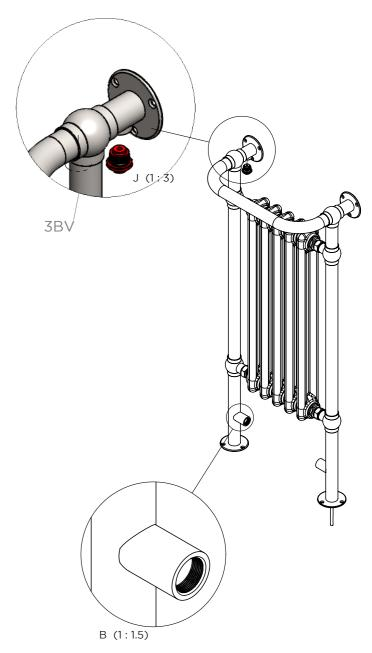
Max.Working Pressure = 8 Bar Max.Working Temprature= 95° C Inlet / Outlet : 1/2" BSP
