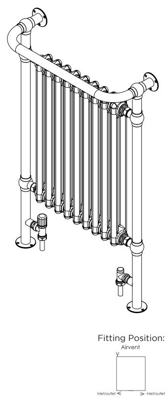
All Dimension are in mm Max.Working Pressure = 10 Bar Max.Working Temperature=95° C Inlet / Outlet : 1/2" BSP
