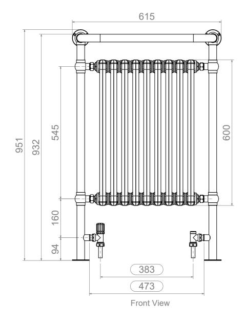
ALL MEASUREMENTS ARE IN MILLIMETRES | MANUFACTURED FROM MILD STEEL
