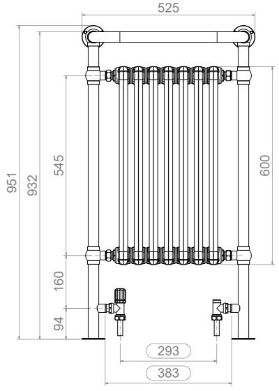
ALL MEASUREMENTS ARE IN MILLIMETRES | MANUFACTURED FROM MILD STEEL
