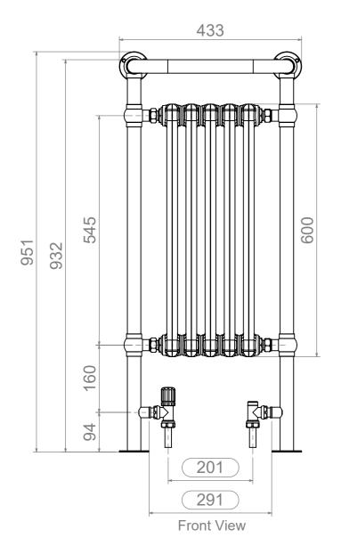
ALL MEASUREMENTS ARE IN MILLIMETRES | MANUFACTURED FROM MILD STEEL
