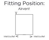
All Dimension are in mm Max.Working Pressure = 10 Bar Max.Working Temperature=95° C Inlet / Outlet: 1/2" BSP
